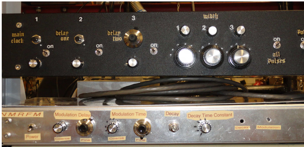
Figure 3.6: This is a picture of the pulse programmer electronics box. It is in black. The modulation box is below it.
