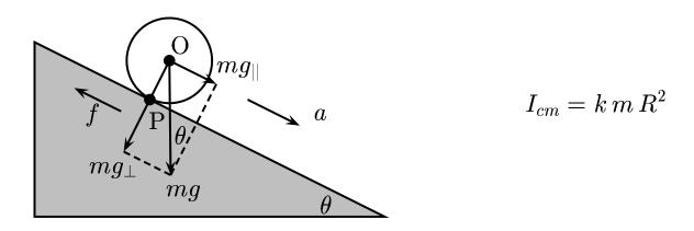
The equation of motion along the incline, " $\tau = I \alpha$ ", is given by
