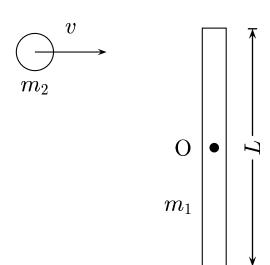
A rod has mass  $m_1$  and length L. It is pivoted at the midpoint. The clay has a mass  $m_2$  and velocity v. It hits the top of the rod and sticks to the rod. It causes the rod-clay system to spin about O. Ignore gravity.
