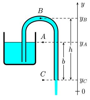
A siphon, which is a flexible tube with a circular cross section, is used to drain water from a tank, see sketch.
