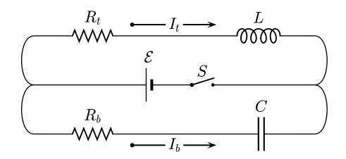
Find  $I_t$ ,  $I_b$ ,  $V_L$ , and  $V_C$  at t = 0, just after switch S is closed.
