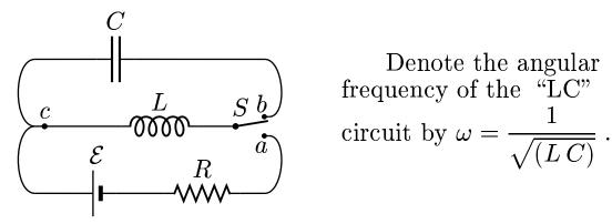
The switch S is left at position a for a long period of time. The switch S is then moved from position a to b at t=0.
