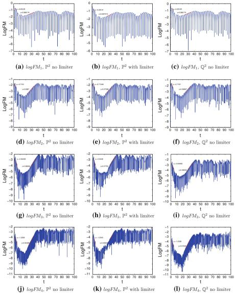
**Fig. 7** Evolution of the first four Log Fourier mode as a function of time for nonlinear Landau damping. Various values of the numerical damping/growth rate are marked on the *graphs*. Here the  $\mathbb{P}^2$  space with the positivity-preserving limiter was used on a  $100 \times 200$  mesh. The predicted recurrence time  $T_R$  for log  $FM_1$  is 209.44, for log  $FM_2$  is 104.72, for log  $FM_3$  is 69.81, and for log  $FM_4$  is 52.36
