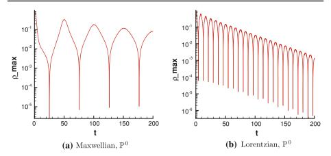
Fig. 1 Computations of the advection equation for piecewise constant polynomials showing local maxima of the density  $\rho_{\text{max}}$  as a function of time. The mesh is  $40 \times 40$  with  $\Delta x = \pi/10$ . For the Maxwellian equilibrium  $\Delta v = 1/4$ , while for the Lorentzian equilibrium  $\Delta v = 3/2$
