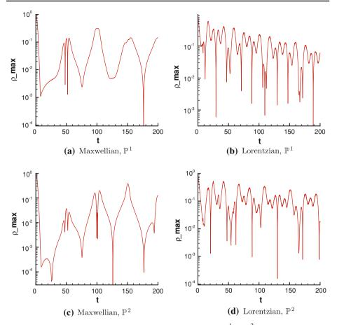
**Fig. 3** Computations of the advection equation for the polynomial spaces  $\mathbb{P}^1$  and  $\mathbb{P}^2$  showing local maxima of the density  $\rho_{\text{max}}$  as a function of time. The mesh is  $40 \times 40$  with  $\Delta x = \pi/10$ . For the Maxwellian equilibrium  $\Delta v = 1/4$ , while for the Lorentzian equilibrium  $\Delta v = 3/2$
