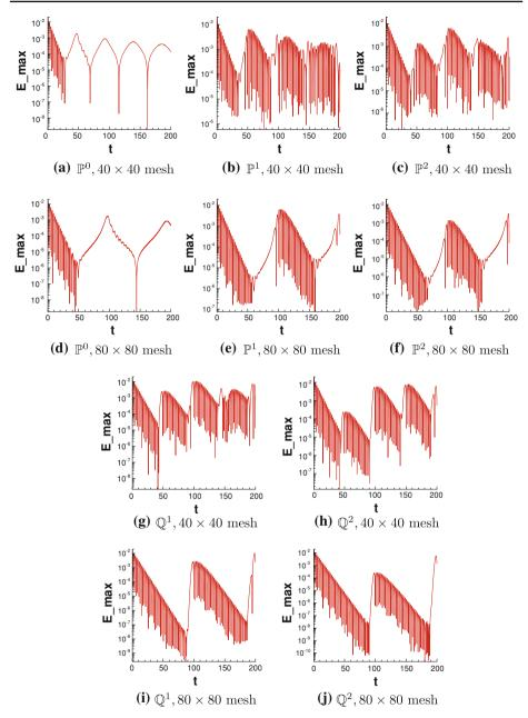
Fig. 4 Depiction of linear Landau damping showing recurrence in the maxima of the electric field,  $E_{\text{max}}$ , as a function of time for various polynomial spaces
