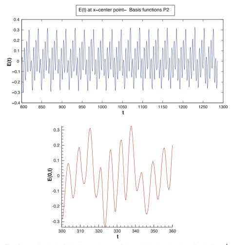
**Fig. 15** (*Top*) The electric field E(0, t) at the center of the spacial domain at later times for the drive  $A_d^A$ . The periodic structure is due to multiple interacting BGK-like states. (*bottom*) Blow up indicating a period-4 modulation of a central hole such as that of Fig. 12). The simulation was done with  $\mathbb{P}^2$  elements with a limiter on a 200 × 400 mesh
