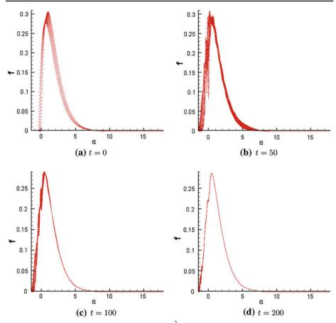
**Fig. 10** Plots of the distribution f(x, v, t) versus  $\epsilon = \frac{v^2}{2} - \Phi(x, t)$  for the two-stream instability at the times *t* indicated, showing saturation to a BGK state. Here the  $\mathbb{P}^2$  space with the positivity-preserving limiter was used on a 100 × 200 mesh
