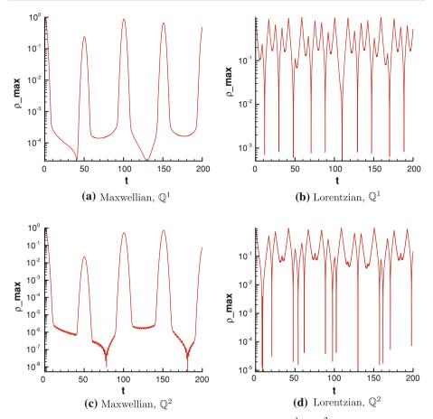
**Fig.2** Computations of the advection equation for the polynomial spaces  $\mathbb{Q}^1$  and  $\mathbb{Q}^2$  showing local maxima of the density  $\rho_{\text{max}}$  as a function of time. The mesh is  $40 \times 40$  with  $\Delta x = \pi/10$ . For the Maxwellian equilibrium  $\Delta v = 1/4$ , while for the Lorentzian equilibrium  $\Delta v = 3/2$
