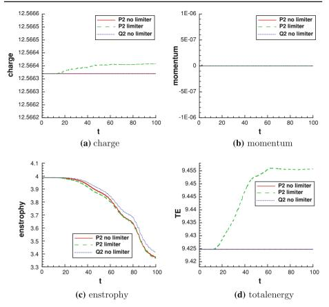
Fig. 8 Evolution of conserved quantities as a function of time during the course of nonlinear Landau damping for various computational methods. A mesh of  $100 \times 200$  was used
