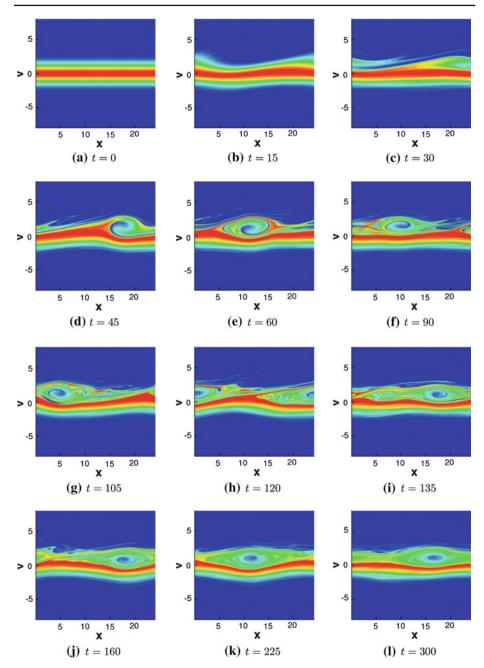
Fig. 14 Phase space contour plots for the KEEN wave at the times indicated. A large amplitude drive of  $A_m = 0.4$  was used, along with the  $\mathbb{P}^2$  basis and a positivity-preserving limiter on a 200 × 400 mesh
