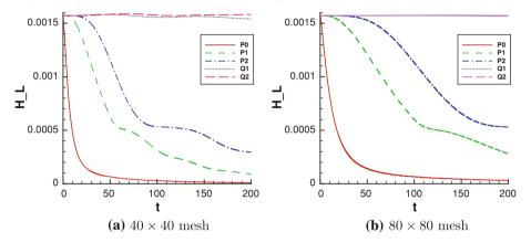
**Fig. 5** Evolution of the linear energy  $H_L$  of (16) as a function of time, while the Vlasov system undergoes linear Landau damping. Various polynomial spaces and mesh sizes were used, as indicated
