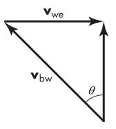
The diagram here shows a boat attempting to cross a river. Assume that the boat's speed relative to the water  $v_{bw} = 10$  m/s and that the current (the water's speed relative to the Earth)  $v_{we} = 5$  m/s.
