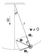
A simple pendulum consists of a string of length r and a ball attached to its end. When the string makes an angle  $\theta$  with the vertical and the tangential velocity of the ball is pointing toward the vertical line, determine the corresponding tangential acceleration:
