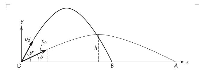
Two projectiles are launched simultaneously and with the same launching speed from point O as shown  $\mathbf{v}_{0'} = \mathbf{v}_0$ . The first is launched at angle  $\theta$  and hits target A in time  $t_A$ . The second is launched at a greater angle  $\theta' > \theta$  and hits target B in time  $t_B$ . Compare the flight times for the two projectiles:
