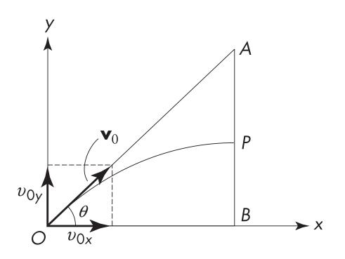
Consider a gun at O aiming at a target located at point A. The gun fires at time t = 0, and at the same time the target begins to fall from rest. Let  $v_{Ox} = 10 \text{ m/s}$  and  $v_{Oy} = 20 \text{ m/s}$ . Also, let OB = 20 m and AB = 40 m. Find the height BP as the bullet passes the vertical line AB:
