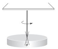
A circular disk is suspended by a wire attached at the top of some fixed support. When the disk is twisted through some small angle  $\theta$ , the twisted wire exerts a restoring torque on the body that satisfies  $\tau = l\alpha = ld^2\theta/dt^2 = -\kappa\theta$ , where  $\kappa$  is referred to as the *torsion constant* of the wire. Find the period of the oscillation:
