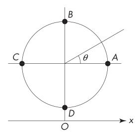
Consider a simple harmonic motion (SHM)  $x = A \cos \theta$  as a projection of a uniform circular motion with  $\theta = \omega t + \phi$ . If at t = 0, x = 0 and  $v = v_0 > 0$ , determine  $\phi$ :
