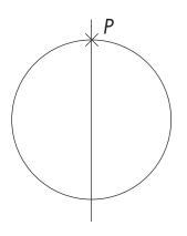
The period of a physical pendulum is  $T = 2\pi \sqrt{\frac{l}{mgb}}$ , where *m* is the mass, *l* is the moment of inertia about the pivot point, and *b* is the distance between the pivot point and the center of gravity. Consider a circular loop oriented vertically where the pivot point *P* is at the top of the loop (see the sketch). Find *b* and *l* for a loop with radius *r* and mass *m*:
