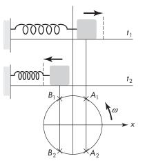
Consider the mass-spring system shown here at two different time  $t_1$  and  $t_2$ , where the mass oscillates according to simple harmonic motion:  $x = A \cos(\omega t + \phi)$ . The motion is modeled as the projection of the circular motion shown at the bottom. Locate the point on the circle that corresponds to the time  $t_1$ :
